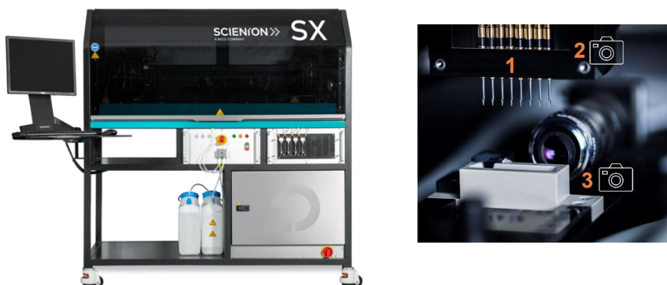
Figure 2: (Left) The sciFLEXARRAYER SX precision dispenser with integrated sciDROP PICO technology used in this study. (Right) Enlarged image of the dispensing unit of the sciFLEXARRAYER SX, including (1) Piezo Dispense Capillaries, (2) the head camera used for imaging targets after printing and (3) the drop high resolution camera allowing to visualize and quantify drop parameters.
