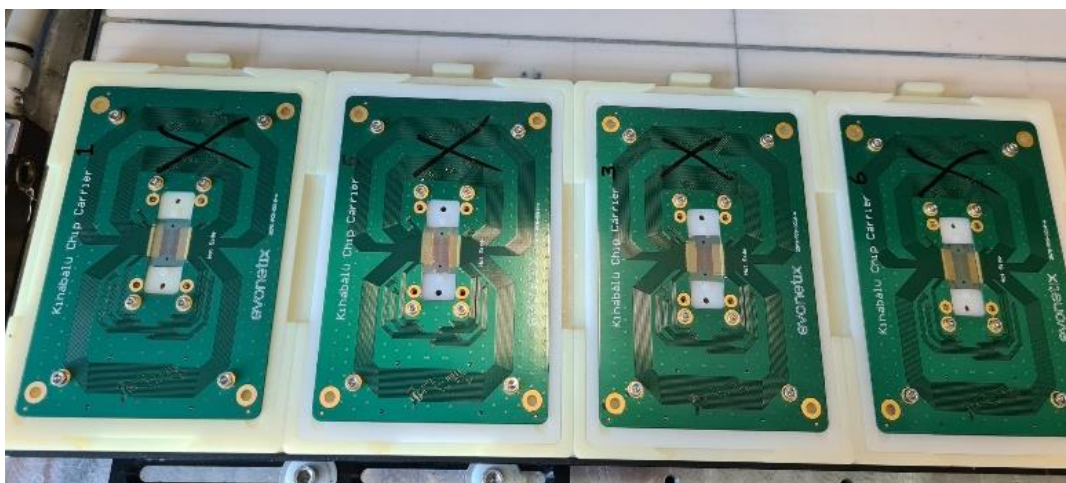
Figure 5: Four Kinabalu chip carriers with coated chips placed on the target deck of the sciFLEXARRAYER SX.
