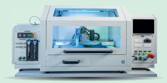
Ultrasonic thin film coating of microtiter plates, biosensors and lateral flow applications
