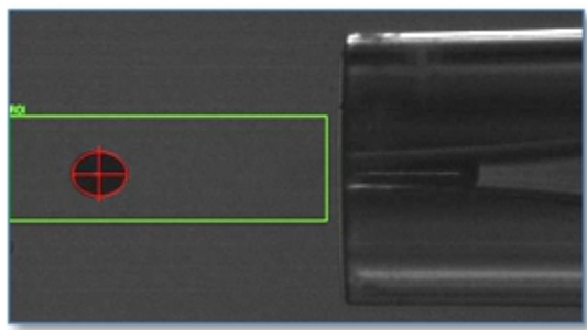
Fig.1 Autodrop detection with calculated drop volume (drop volume 350pl)
