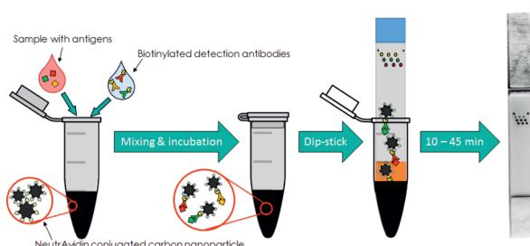
**Fig. 3** Overview of the half-stick assay format chosen for assay development. After mixing and incubation of the sample containing target analytes with biotinylated detAb and NeutrAvidin-functionalized black nanoparticles in optimized running buffer, the half stick is incubated in 100  $\mu$ L thereof. The half stick lacks a sample pad and only carries a non-loaded conjugate pad for submerging into the test mix.
