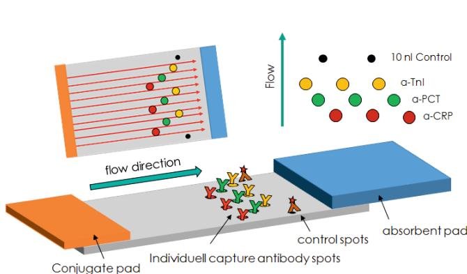
**Fig. 2** Schematic representation of a perfectly staggered multiplex microarray pattern printed onto LFA strips. Triplicates are arranged perpendicular to the flow. The  $3 \times 3$  array is shifted such way that laterally flowing assay components are only passing a single capture zone avoiding unintentionally influencing assay results caused by depletion and interference. Schematic presentation of printed pattern is shown.
