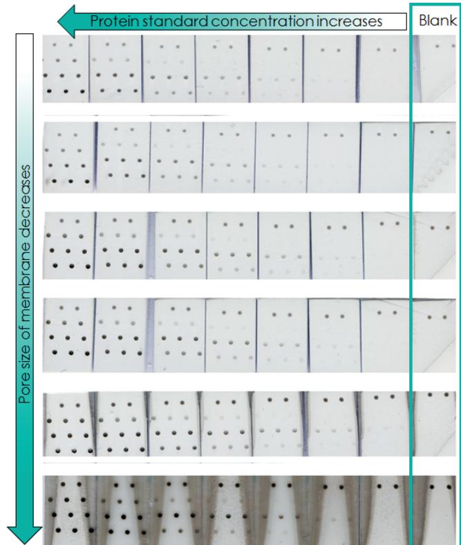
**Fig. 4** Assay performance in dependence of the nitrocellulose flow rate. 10 nL cAb were deposited per spot on membranes varying in flow rate (max and min of the range).
