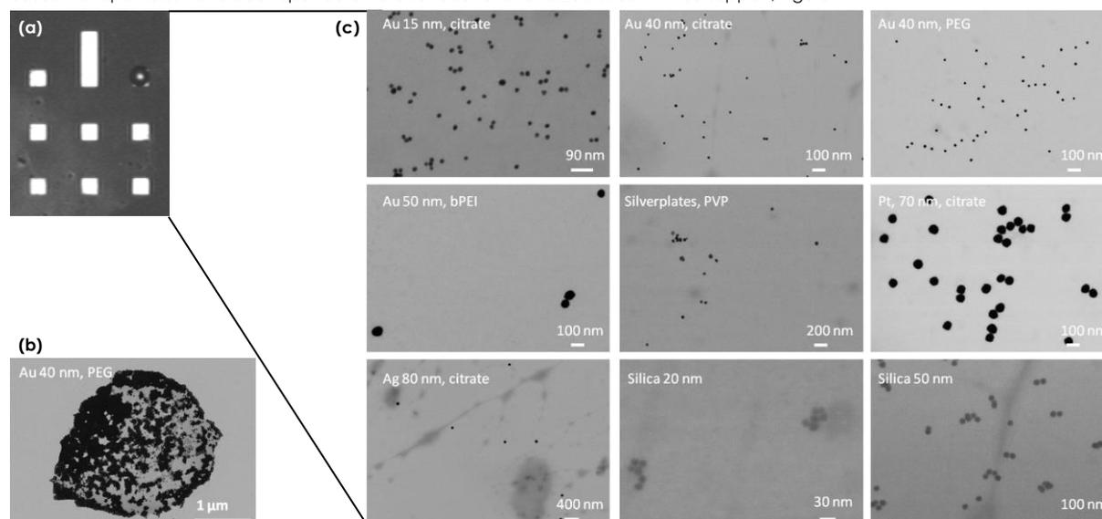
**Figure 1.** SEM images (transmission mode) of different nanoparticle samples on a surface functionalized silicon nitride TEM support (eight windows 100x100 μm and one window 100x350 μm with a membrane thickness of 50 nm; SIMPore).
