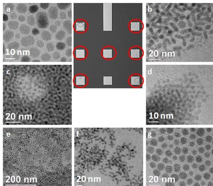
**Figure 1.** TEM images of different samples on a sample grid with silicon nitride membrane (SIMPore TEM grid) a)  $\text{NaYF}_4 < 100\text{ nm}$  b)  $\text{CdTe } 3 \times 10\text{ nm}$ ; c)  $\text{CdSe } 4\text{ nm}$ , diluted d)  $\text{CdSe } 3 \times 10\text{ nm}$ ; e)  $\text{CdSe } 4\text{ nm}$  undiluted f)  $\text{NaYF}_4 9\text{ nm}$ ; g)  $\text{NaYF}_4 < 100\text{ nm}$ .
