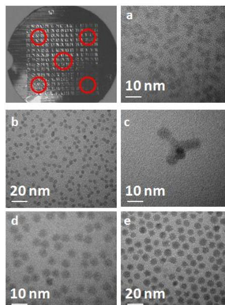
**Figure 2.** TEM images of different samples on a copper grid with carbon film (Ted Pella Inc.) a)  $\text{CdSe } 4\text{ nm}$ ; b)  $\text{CdSe } 6\text{ nm}$ ; c)  $\text{CdTe } 3 \times 10\text{ nm}$  d)  $\text{NaYF}_4 9\text{ nm}$ ; e)  $\text{NaYF}_4 6\text{ nm}$ .
