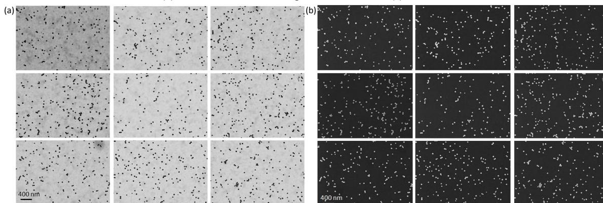
**Figure 2.** SEM images of bPEI stabilized gold nanoparticles on a functionalized grid with silicon nitride membrane (SIMPore), (a) transmission mode, (b) in-lens-detection.
