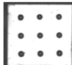
**Figure 1.** Spotted array of nine replicates on a 1x1 mm silicon nitride membrane.
