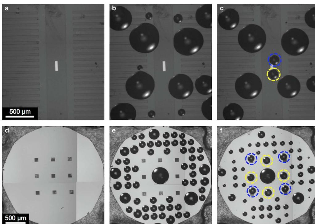
**Figure 1.** Optical images of Hummingbird Scientific 200 nm spacer-chips with a single 50 nm thick,  $200 \times 50 \mu\text{m}$  window (a–c) and a Norcada 10 nm thick  $100 \times 100 \mu\text{m}$ , nine window array (d–f), showing the windows predeposition (a,d), postdeposition of pure water to create a high-humidity environment (b,e) and postdeposition of 20 nm gold nanoparticles (yellow) and 200 nm UiO-66 (blue) (c,f).
