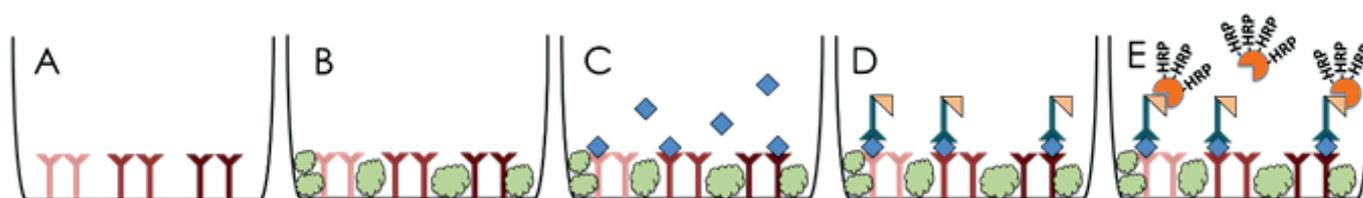
**Fig. 1** Schematic procedure of the stepwise sandwich ELISA. Printing or coating of capture antibodies in sciPLEXPLATES Type1 (A) . (B) SCIENION's optimized blocking procedure. Investigation for sensitive quantification incubation protocols for (C) analytes and (D) biotinylated detection antibodies. Using Streptavidin-PolyHRP conjugate for increasing the LOD (E). A customized washing procedure with sciWASH Protein D1 between steps (B) to (E) is necessary.
