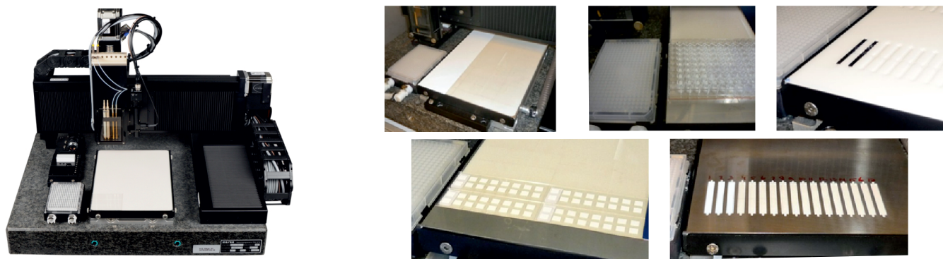
Fig. 2 sciFLEXARRAYER S3; Examples of surfaces onto which binding proteins are being printed (from left to right and top to bottom): Nitrocellulose membrane sheets, ELISA plates with transparent or non-transparent bottom, biosensor chips in a Delrin template, slides with nitrocellulose pads and nitrocellulose lateral flow membranes for microarray applications in a metal template.
