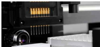
sciFLEXARRAYER dispensing head with horizontal camera for drop volume measurement and vertical camera for online control of printed arrays in microtiter plate
